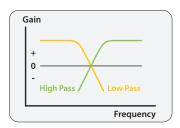
The characteristics of the filter change in the extreme positions of the EQ Gain controller: the fully counter-clockwise setting will produce a low pass filter; fully clockwise position will result in a high pass filter. The overall level can drop quite noticeably then, but this can be corrected with the gain controller easily.
