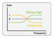
Its main function is to change the proportions between high and low frequencies. The principle is quite similar to a pair of scales: Dependent on the gain setting around a variable center frequency, the high frequencies are boosted whereas the low frequencies are attenuated (or vice versa).
