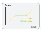
Loud parts in an arrangement can keep their dynamics, as they will not be compressed beyond the limit of the Gain Reduction Limiter. Some very nice special effects like ducking or upward compression can be achieved with it easily by only reducing the quieter parts without changing the original dynamics at the same time.
