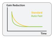
This is where the Auto Fast function comes into play. For example, if you set the attack to 80 ms and then engage the Auto Fast mode, the attack time will be shortened automatically on fast and loud signal impulses. The compressor reduces the signal quickly and prevents it from slipping through.
