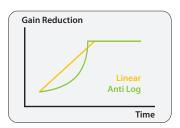
But if intentionally striking and creative compression as well as producing new and interesting sounds are the sought-after goals, it definitely makes sense to turn the established approach upside down. For this reason, you can switch the release curve of the mpressor from linear to antilogarithmic.
