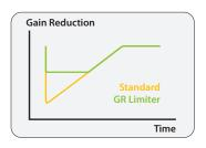
For comparison, just imagine a fader on a mixing console with your hand moving the fader to 'play compressor'. If now the fader was limited by a piece of duct tape at 10 dB, for example, it could only reduce the signal up to this value. If the input level dropped below this limit, the fader would be moved up correspondingly.
